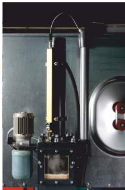
Position sensor for controlling the operations of the cylinder and the form. In addition, the central lubrication system
