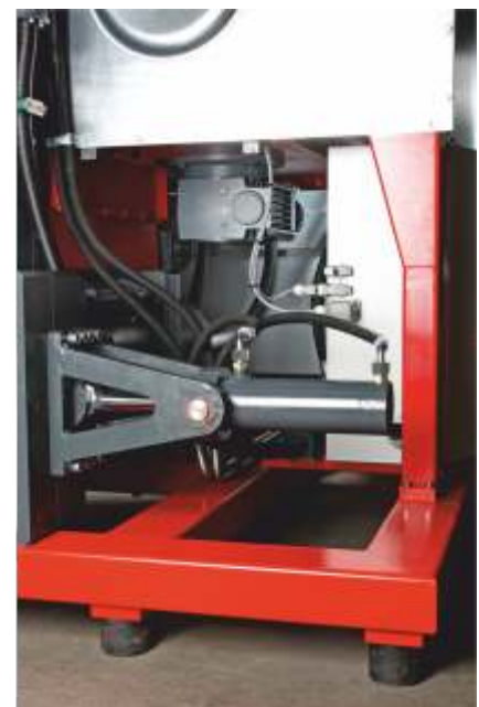
Powerful hydraulic cylinders, gear motors for the agitator and screw conveyor
